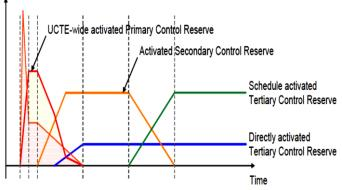
Fig. 2. The principle of mobilizing power reserves
